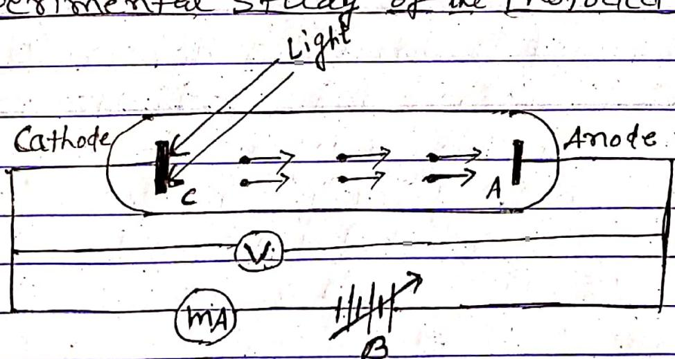
This fig. consists of an evacuated glass or quartz tube with two electrodes. The photosensitive surface forms the cathode. A potential difference is maintained between the cathode C and anode A by a variable battery B. The photoelectric current is measured by a milliammeter (mA) while potential difference
