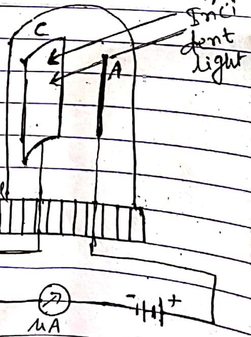
in the form of a wire so that it does not obstruct the light falling on the cathode.
